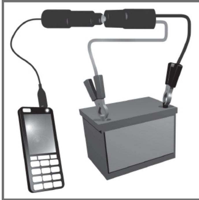
Recharging portable devices with a large battery
