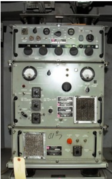
One of the Battleship Iowa 's AN/URT-23(C) transmitters. The exciter is at the top, the PA is in the middle, and the amplifier power supply is on the bottom. [Jim Jerzycke, KQ6EA, photo]
